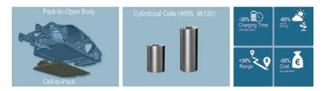
**Fig. 8.11** BMW's Gen6 battery cell and pack architecture and the resulting improvements of some relevant KPIs (the reference is the present Gen5 battery pack architecture)
