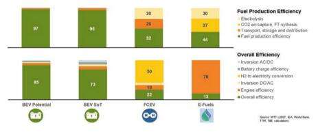
**Fig. 8.7** The efficiency of different powertrain options (*BEV* Battery Electric Vehicle, *SoT* State of Technology, *FCEV* Fuel Cell Electric Vehicle) (own illustration based on European Federation for Transport and Environment (2017))
