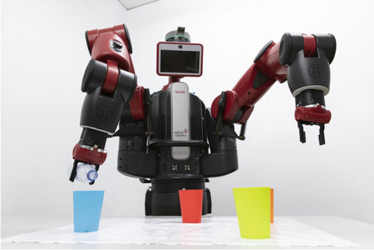
Fig. 2 Baxter robot for small factories
