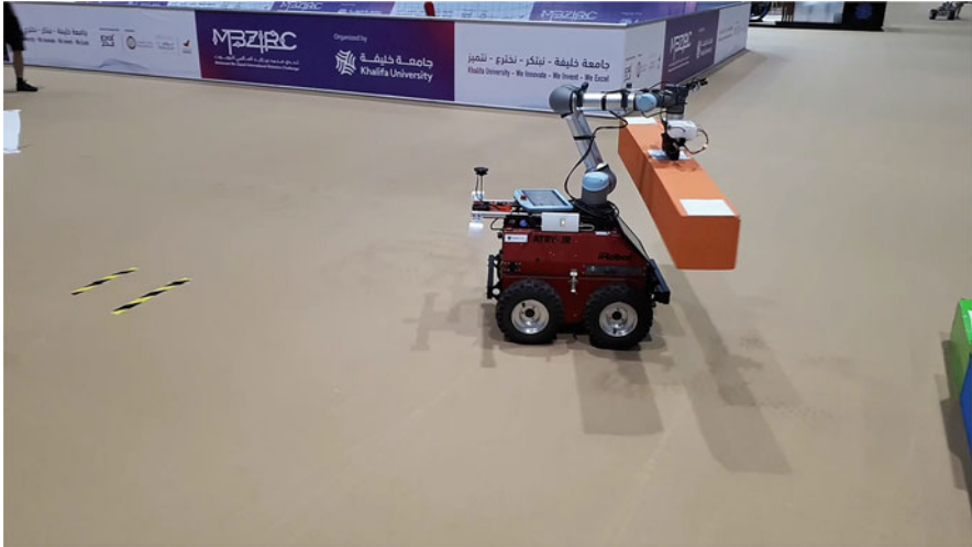
Fig. 1 Service robot for construction and brick transportation
