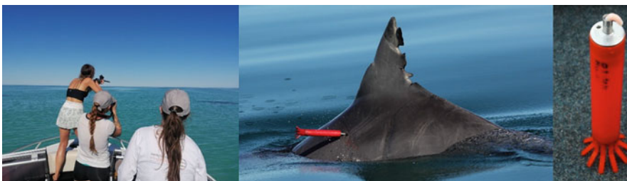
Fig. 2.1 A skin sample is collected from a bottlenose dolphin in Shark Bay using a modified rifle (left panel). The biopsy dart penetrates the skin and then bounces free of the animal while retaining a skin sample (middle panel). The dart consists of a steel tip holding the skin sample and a floating polycarbonate body that permits easy sample recovery at sea (right panel). Image credit: Shark Bay Dolphin Project, Svenja Marfurt (left panel), Samuel Wittwer (middle and right panel)
