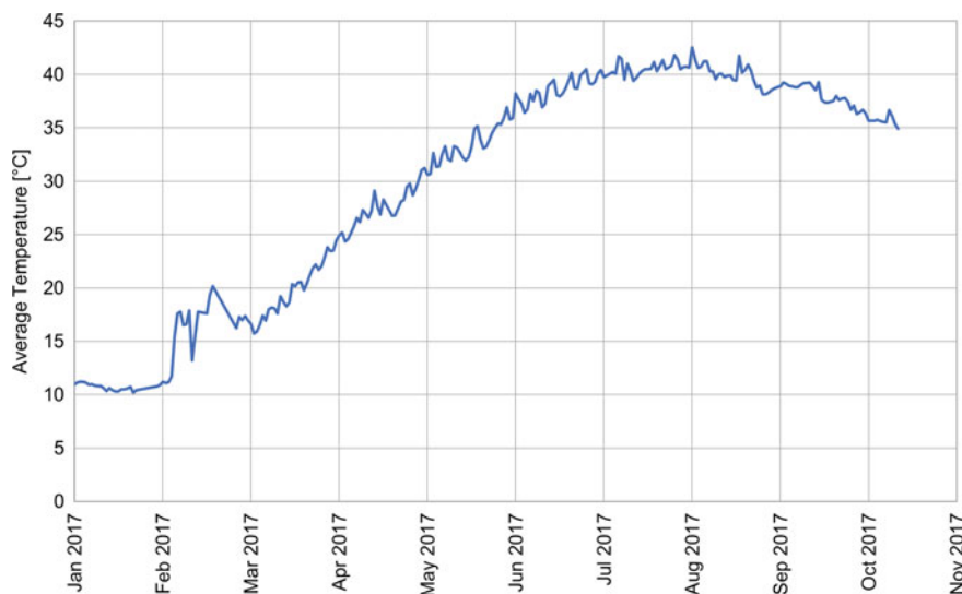
Fig. 18.14 Thermally enhanced bioremediation TCH low-temperature heating progression
