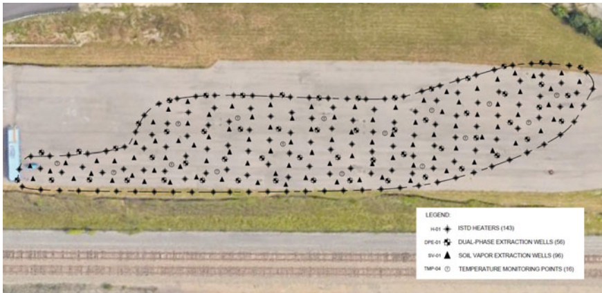
Fig. 18.13 Low-temperature heating via thermal conduction heating for thermally enhanced bioremediation of hydrocarbons-Schenectady, New York
