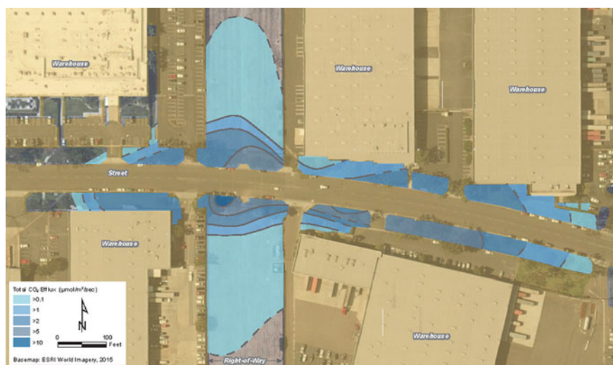
Fig. 13.1 Site A: illustration of CO 2 efflux at site with pervious and impervious ground cover (blue shading indicates areas where CO 2 efflux occurs over pervious ground cover areas and was included in the geospatial integration to estimate the sitewide NSZD rate)
