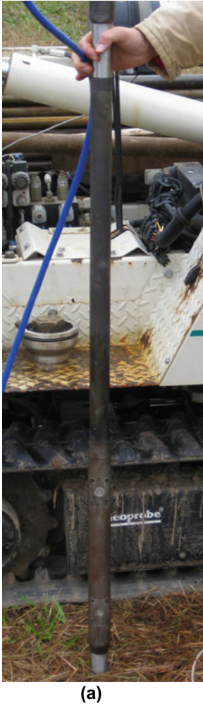
Fig. 7.9 Prototype HRK tool: a Picture showing the bottom injection screen with the two pressure transducers inset into the rod above the screen, and b expanded view of the pressure transducer screen. Water is injected through the bottom screen and both transducer ports during probe advancement
