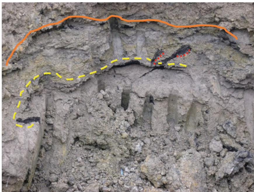
Fig. 16.1 Excavation post-CBI emplacement in the vadose zone demonstrates significant horizontal distribution. The CBI contained PAC. Note the horizontal carbon sheet above the bucket mark traced by a yellow line (dashed). The carbon sheet was ~1.2 m across. A shallower horizontal sheet is traced by an orange line (solid). Two angular carbon sheets having more vertical character are marked by red lines (dotted)
