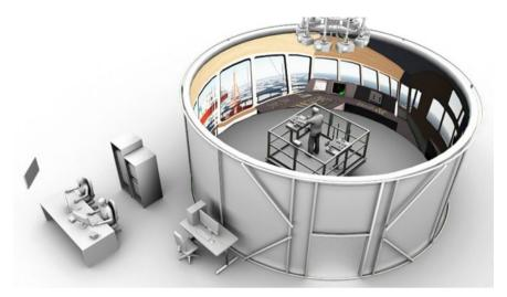
Fig. 7.4 Ship simulator setup
