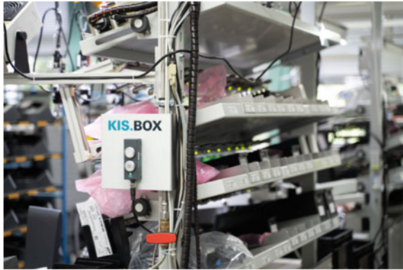
Fig. 3.28 Sample KIS.BOX installed at the assembly station
