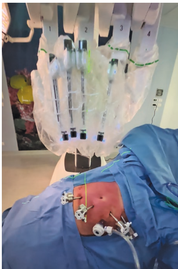
Fig. 16.2 Driving the laser lines to the scope port
