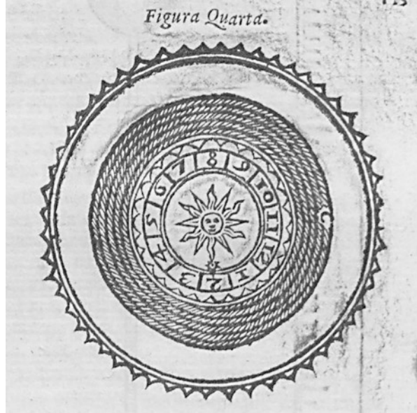
Fig. 7.20 Second version of a hygrometer, modeled on a clock (Sanctorius 1625: 23, 215). (© British Library Board 542.h.11, 23)
