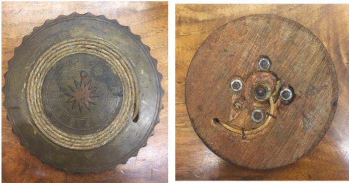
Fig. 7.21 Replica of Sanctorius's clock type of hygrometer. (The replica was made by Loris Premuda for an exhibition held in 1961 at the University of Padua, where it can still be found today. The replica is imperfect, however, since the cord is affixed to the disc by glue and nails, and is thereby prevented from contracting or loosening (Biblioteca medica 'Vincenzo Pinali antica' dell'Università degli Studi di Padova, © Philip Scupin))
