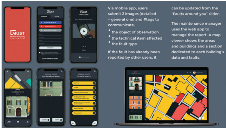
Fig. 18.1 From the mobile app to the facility manager dashboard workflow. Authors elaboration
