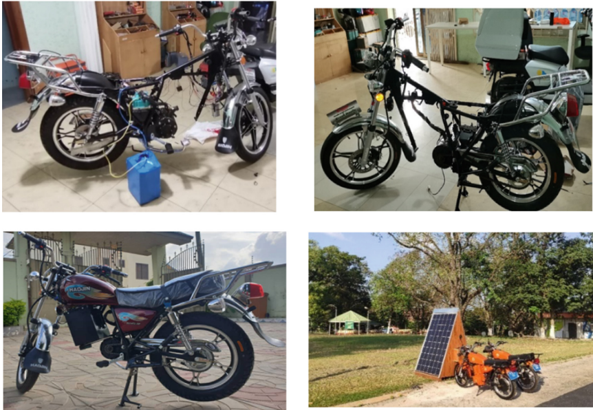
Fig. 2. a. Conventional motorbike stripped internal combustion engine (top right, Model: Haojin 125–32, 150cc). b. Rewired conventional motorbike linked to a battery pack (top left). c. Fully converted ICE motorbike at the campus of UENR (Left)(original model was Haojin 125–32, 150cc). d. E-mopeds and stand-alone solar charging stations on the campus of KNUST (Right).
