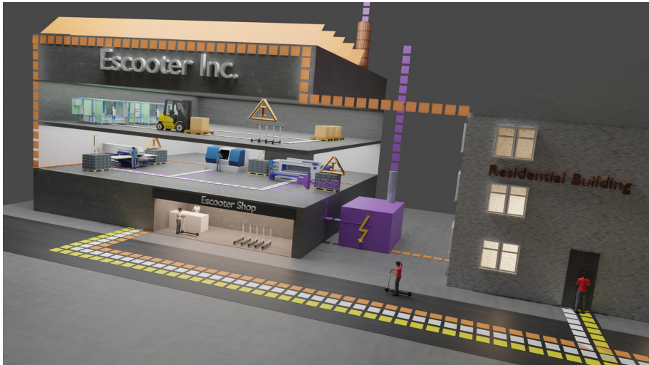
Fig. 1. Mockup of an AR UP scene with production and distribution close to the customers. In the scenario, both interconnection (highlighted purple emissions, orange energy, yellow people, white material) and value stream planning combined with sector coupling (utilisation of process heat and excessive energy for private residences) are based on [16]
