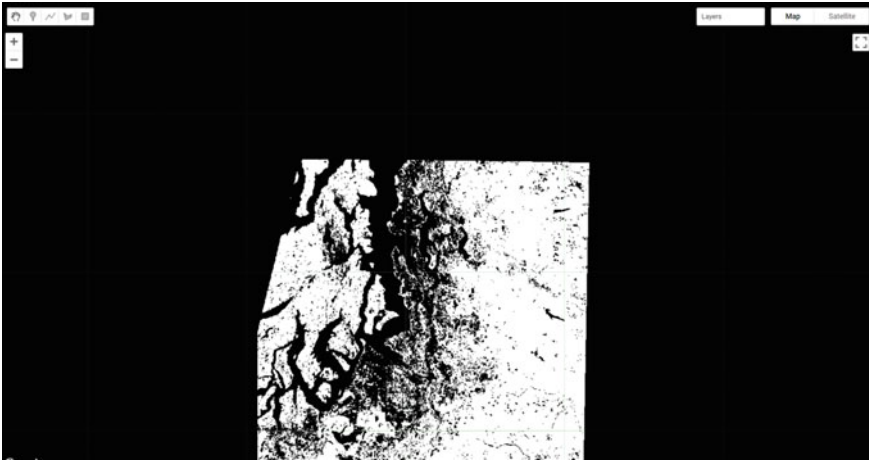
Fig. 5.11 Updated mask. Areas of non-forest are now masked out as well (black areas of the image)
