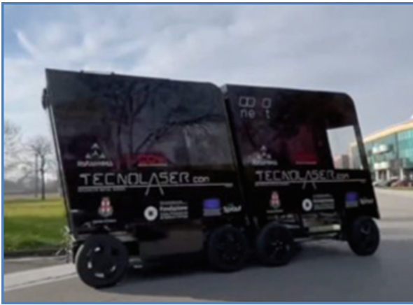
Fig. 1. Run session trial with two paired electric autonomous pods (NEXT system) for cargo hitching in Padua (SPROUT project)
