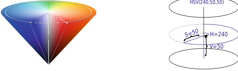
Fig. 3. HSV color model: On the left, the cone of possible colors for various hue color angles H , saturations S , and darkness values V are shown. H can take values between 0^\circ and 360^\circ , S and V between 0 and 100. The example of how to compose the color “navyblue” in this HSV color model is presented on the right. (pictures taken from wikipedia [29]) (Color figure online)
