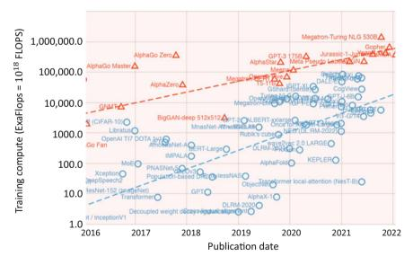
**Fig. 8.3** Around 2016, a new trend of very large models emerged (red). These were developed by leading Internet companies that were able to finance the investment. The lower blue line illustrates the average computational effort of regular models, e.g. from universities. Note the logarithmic scale of the training compute. Image cutout from [76, p. 5]
