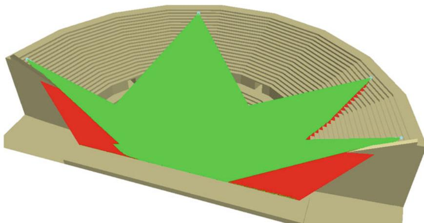
**Fig. 3** Lines of sights built from the observer points in the seating area and the target line on the stage (model N.1). The green lines correspond to visible trajectories and the red lines correspond to non-visible trajectories
