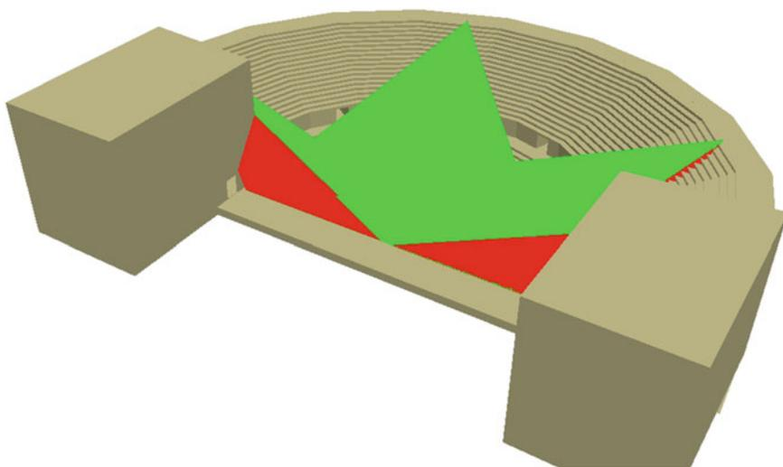
**Fig. 4** Lines of sights built from the observer points in the seating area and the target line on the stage (model N.2). The green lines correspond to visible trajectories and the red lines correspond to non-visible trajectories
