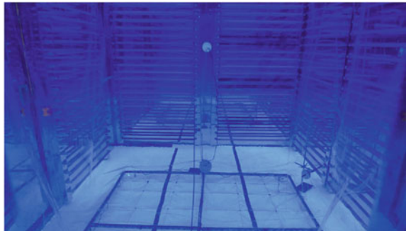
Fig. 1.14 FORTH chamber, a Teflon chamber with side wall illumination
