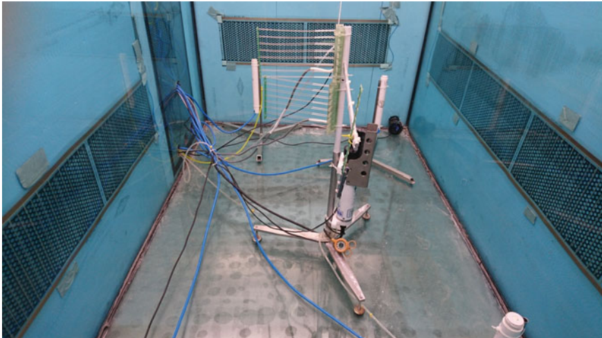
Fig. 8.13 Picture of tank with heating pads placed outside the glass, which is our preferred method, and instrumentation mounted on poles. (Picture from Roland von Glasow Air-Sea-Ice Chamber, Centre for Ocean and Atmospheric Sciences, University of East Anglia)
