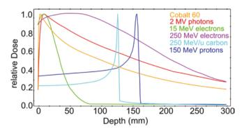
**Fig. 6.1** Comparison of the relative depth dose distribution of 15 MeV electrons (green), 250 MeV electrons (purple), 2 MeV photons (red), 150 MeV protons (dark blue), and 250 MeV/u carbon (turquoise) and cobalt 60 (orange)
