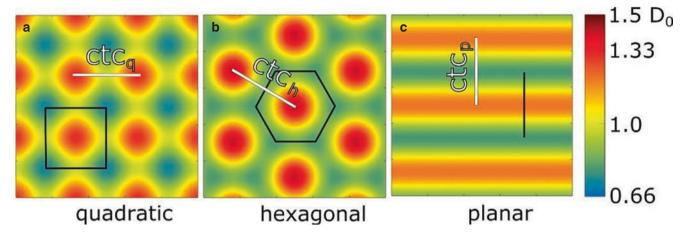
**Fig. 6.12** Quadratic (a) and hexagonal (b) pencil minibeam and planar minibeam (c) arrangements on a 2D lattice with view direction in the direction of the beam. The dose is color coded and normalized to a
