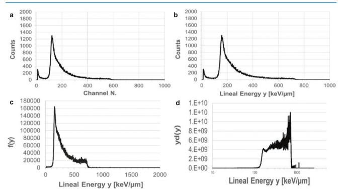
**Fig. 4.11** The same microdosimetric spectrum represented through the raw counts per channel acquired ( $\mathbf{a}$ ), counts as a function of the lineal energy (y) after a channel calibration ( $\mathbf{b}$ ), converted into lineal energy frequency ( $\mathbf{c}$ ) and dose ( $\mathbf{d}$ ) distributions
