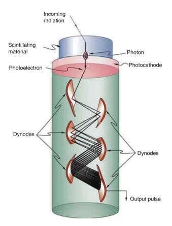
**Fig. 4.5** Schematic diagram of a photomultiplier tube (PMT) (courtesy of Physics Libretexts, Fig. 31.2.3)
