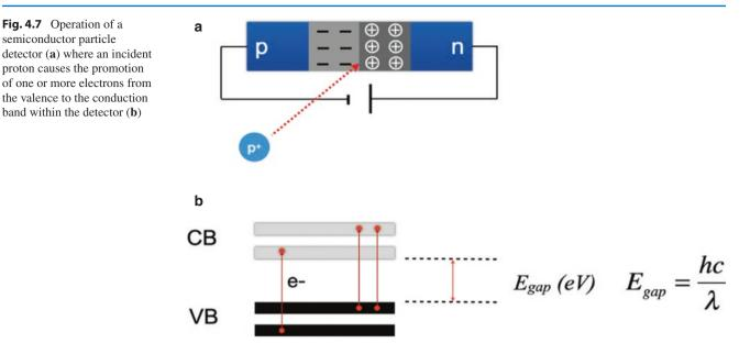
detector. Here, the valence band is equivalent to the energy level of the outermost electron, while the conduction band is the energy level of the next vacant energy state above the valence band. A current is produced which is proportional to the energy loss by the charged particle or photon within the depletion layer [6, 7]
