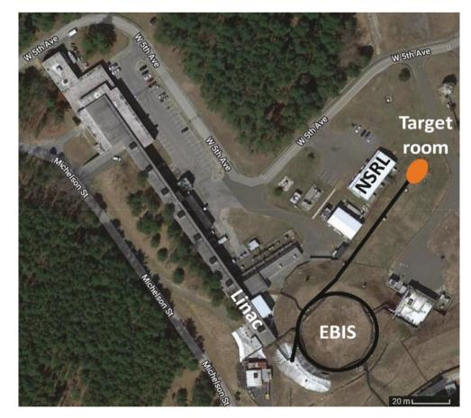
Fig. 10.29 Aerial view and general layout of the NASA Space Radiation Laboratory (NSRL) facility in Upton, NY, USA. *EBIS* electron beam ion source. (Satellite view courtesy Google Earth) Heavier ions with atomic numbers up to Z = 79 (Au) are limited to approximately 350–500 MeV per nucleon (https://www.bnl.gov/nsrl/).
