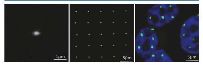
**Fig. 4.15** Proton microbeam with a size of 0.8  $\mu$ m (fwhm) visualized by a fluorescent nuclear track detector. Array of proton micro-beams with a point distance of 5  $\mu$ m in both directions. 53BP1 accumulation in
