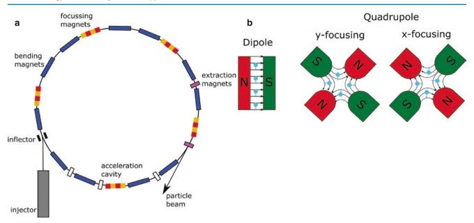
Fig. 6.31 (a) Principle of a synchrotron. (b) A positively charged beam coming from the front is deflected by Dipole magnets and focused by quadrupole magnets
