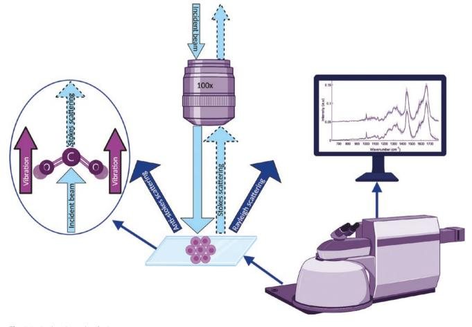
Fig. 7.7 Basic schematic of a Raman spectrometer
