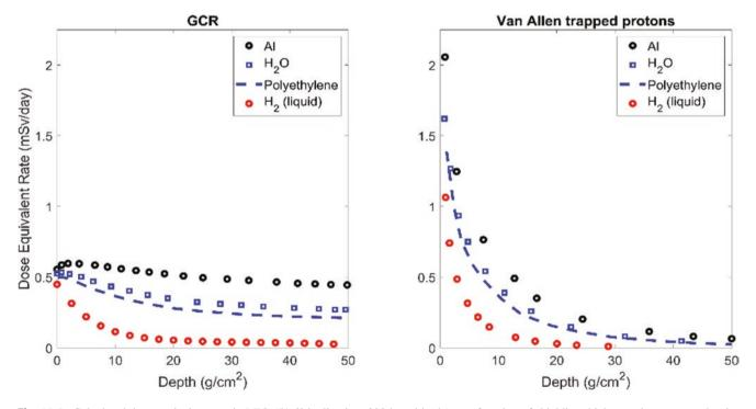
**Fig. 10.9** Calculated dose equivalent rate in LEO (51.6° inclination, 390 km altitude) as a function of shielding thickness given as area density for different shielding materials: (left) GCR, (right) Van Allen trapped protons. (Data used with permission from Dietze et al. [37])
