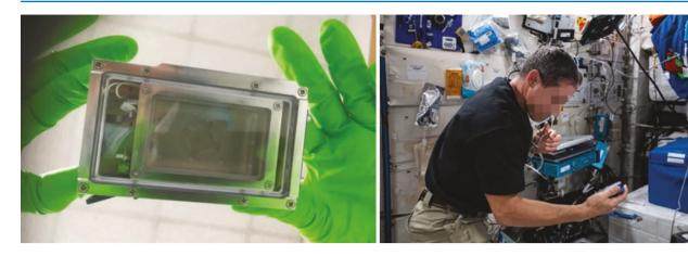
**Fig. 10.21** View of one Rob2 hardware used onboard of the ISS (left) and Astronauts checking the correct rehydration of *A. vaga* individuals. Sixteen pieces of hardware were sent to ISS, each containing 40,000
