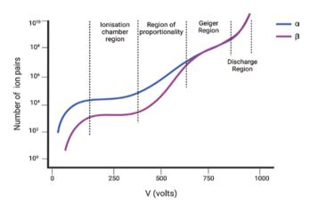
**Fig. 4.3** Signal response to ionization as a function of the applied voltage for heavily ionizing (top curve) and weakly ionizing particles (lower curve). In the Geiger region, the output does neither depend on the voltage nor on the amount of deposited energy or initial ionization. [Adapted from Fig. 4.12 Martin and Shaw (2006). Copyright (2006), Wiley Publishers]
