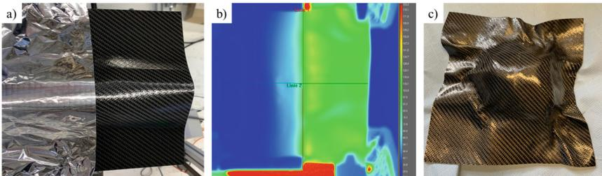
**Fig. 5.** a) Clamped organo sheet with aluminum foil shield, b) Resulting temperature distribution during infrared heating, c) Generated hemispherical frustum
