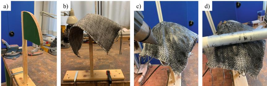
**Fig. 6.** a) Pole & 2D quarter circle tool, b) Commingled weave fixed to the pole, c) Heating with hot air gun, d) Forming, impregnation & consolidation with a roller
