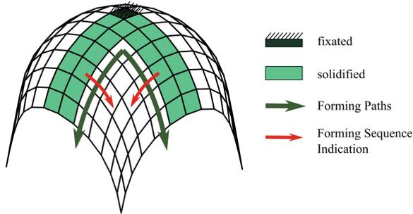
**Fig. 1.** Forming paths & forming sequence for a hemisphere
