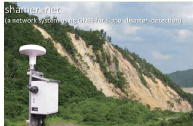
Fig. A.44 “Shamen-net” is a total monitoring system integrating GNSS and other monitoring device (Measurement precision: \pm mm, on a real time basis)
