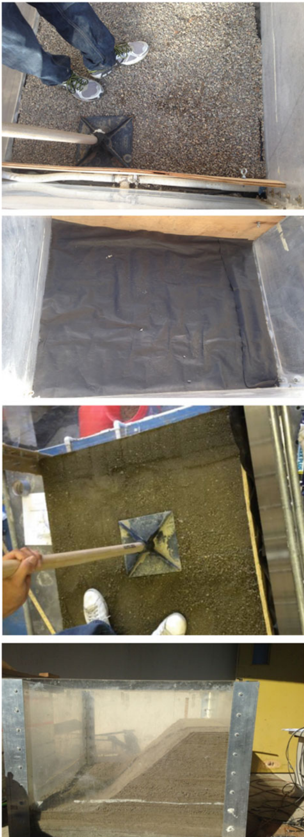
Fig. 1 Process for the preparation of experimental model slopes
