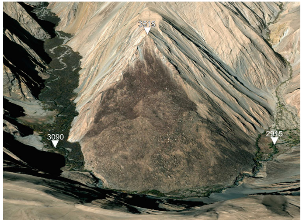
Fig. 10 Rockslide dam in Chinese Pamir and completely silted and forested dammed lake
