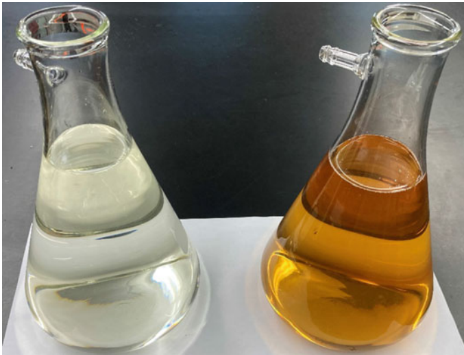
Fig. 29.2 Lake water with low (left) and high (right) concentrations of dissolved organic matter. Photo credit Guillaume Grosbois
