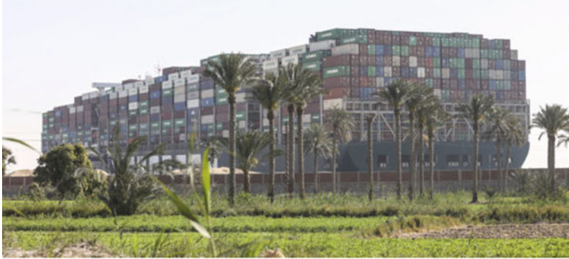
Fig. 9 Cargo stacked 14 stories high on the “Ever Given” 14
