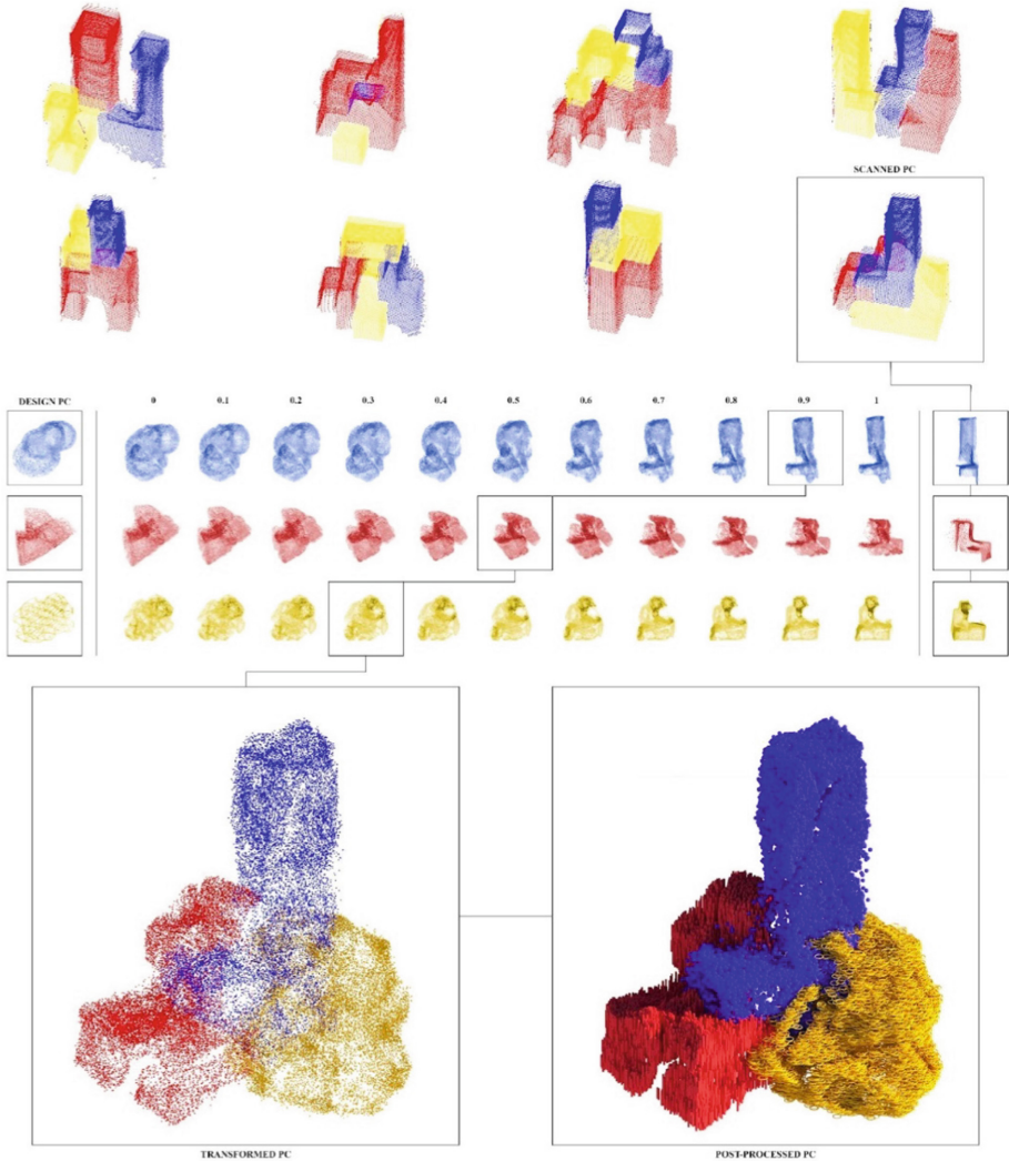
Fig. 7. Top: Variation of scanned concepts for a tower design. Middle: Transformation toward selected design point cloud via autoencoder. Bottom left: Outcome of the transformation. Bottom right: Post-processed point cloud in Unity. The depicted process is running in real-time and is responsive.
