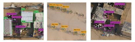
Fig. 4. Examples of missed detections that result from the YOLO-V3 CNN, trained for multi-class object detection
