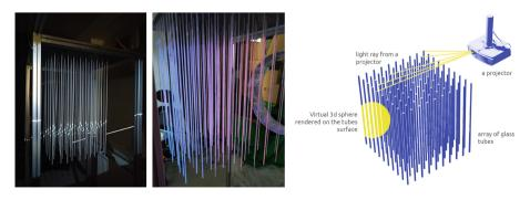
Fig. 4. 3D glass tube display prototype with one video projector as a light source.
