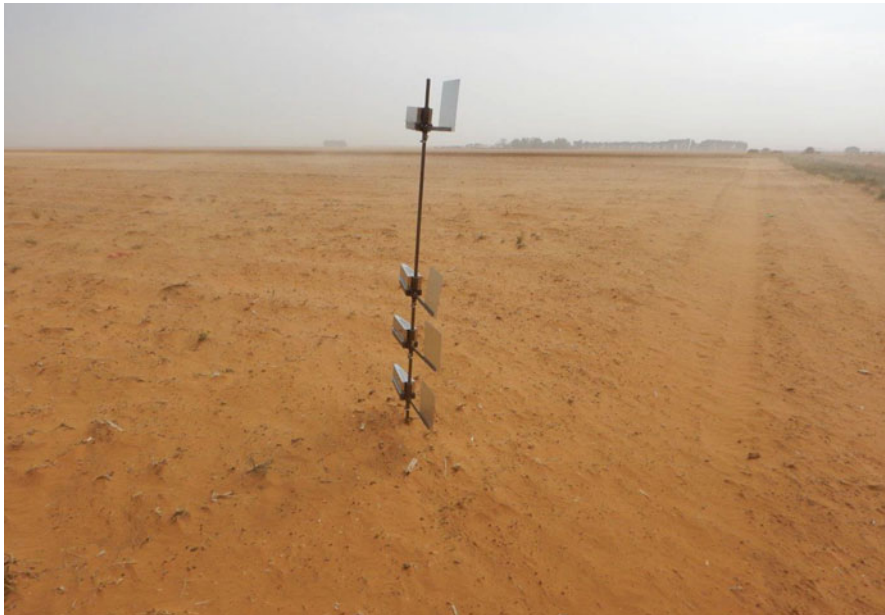
Fig. 13.3 Dust event near Bultfontein, Free State Province. Dust traps are collecting saltating and suspended sediments originating from a bare peanut field in August 2018. PM_{10} concentrations peaked at 2500 ppm during this two-hour event and resulted in the collection of 26 grams of sediment from the 4 traps (Photo: F. Eckardt 2018)
