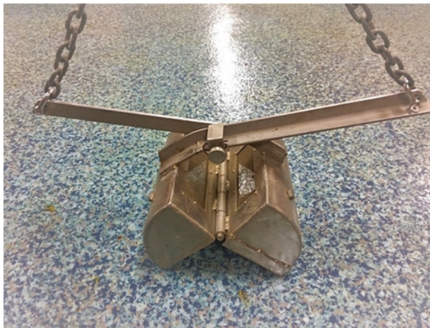
Figure 2.4 A Van Veen grab sampler shown open. Photo: A. Reichelt-Brushett
