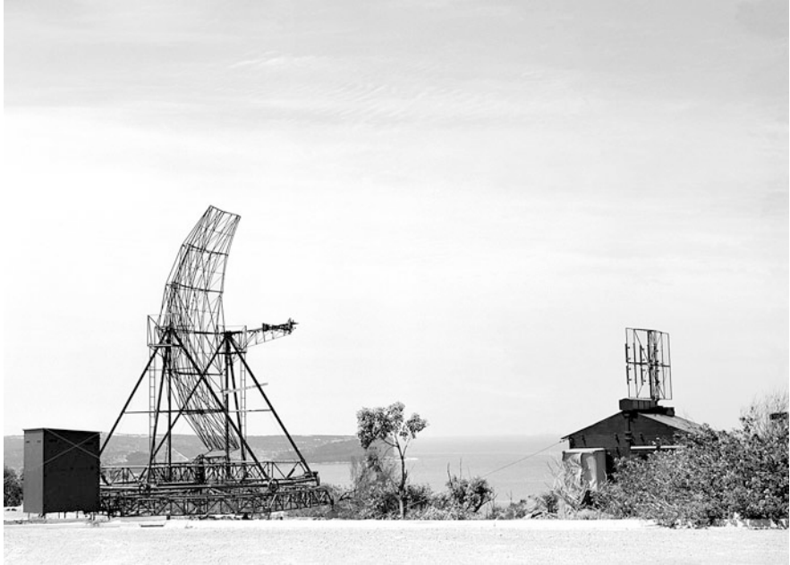
Fig. 9.5 The prototype LW/AWH Mk II. Goss and McGee, 2009, page 60. Both the figure in the Goss and McGee volume and the CRAIA image are reversed left to right. Here the orientation has been corrected. Credit: CSIRO Radio Astronomy Image Archive B1362
