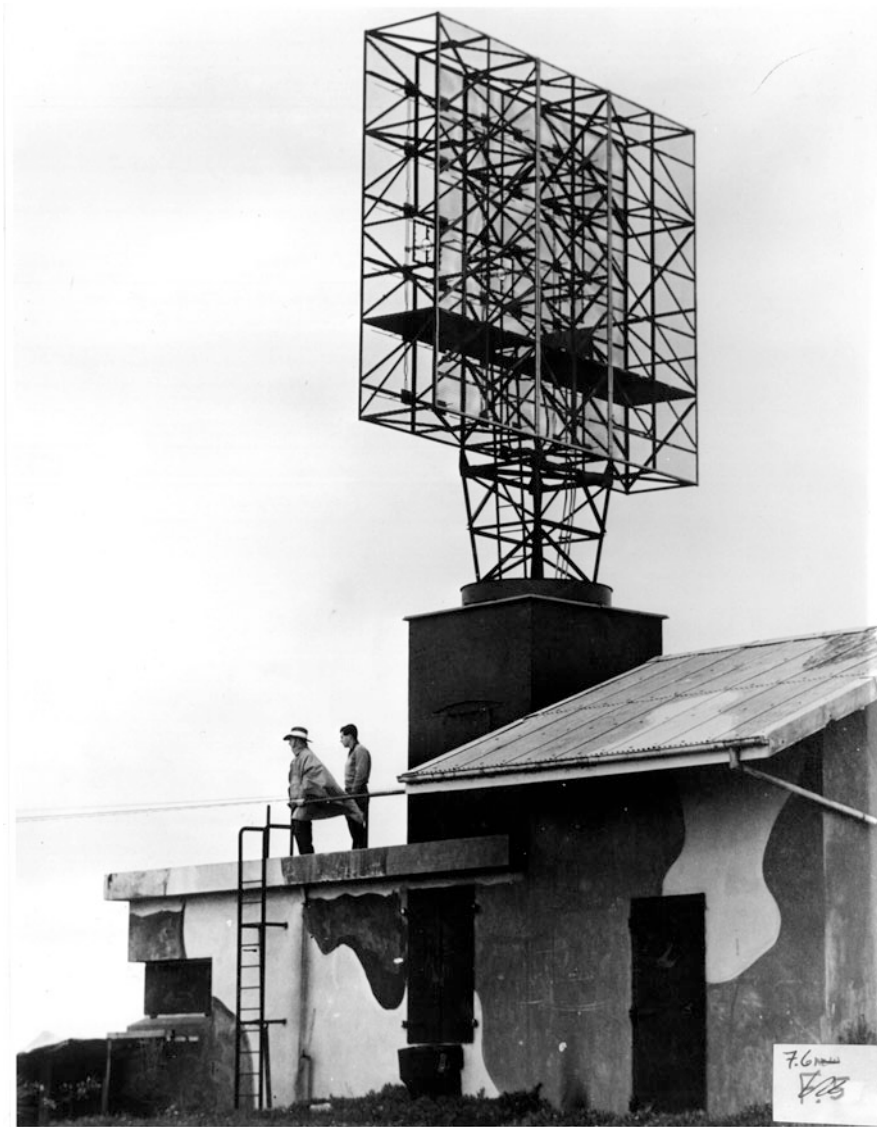
Fig. 13.1 The Shore Defence 200 MHz aerial during WWII. Elevation above the sea was 85 m. Used in January 1946 for the first radio astronomy interferometry of the sun on Australia Day (26 January); the small size of the radio emission (Type I burst) indicated a brightness temperature in the range 0.5 to 100 million K. Credit: CSIRO Radio Astronomy Image Archive JP13-1
