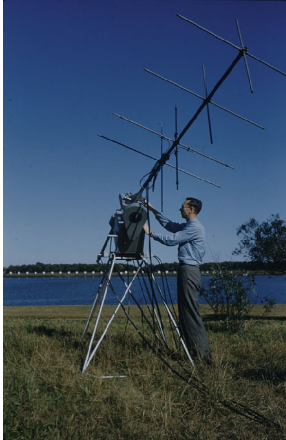
Fig. 16.3 Fritz Goro photo of Pawsey at Potts Hill in March 1951, 98 MHz yagi antenna at the north end of the reservoir. It was used for total power observations of solar bursts. Note the grating array aeri-als (10 foot diameter, used at 20 cm) to the south. Credit: Getty Images, Fritz Goro, The Life Picture Collection , licensed by Getty November 2021/ Licence organised by Shutterstock, Inc., New York, NY (5 Nov 2021) Original, Premium Editorial All Media
