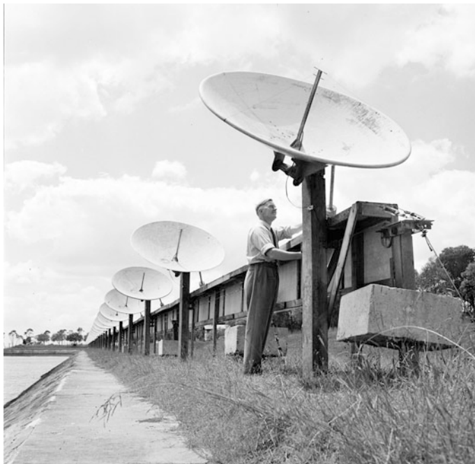
Fig. 37.9 (Chris) Christiansen and his 32-element solar array at Potts Hill Reservoir 1953. Credit: CSIRO Radio Astronomy Image Archive 2976-1
