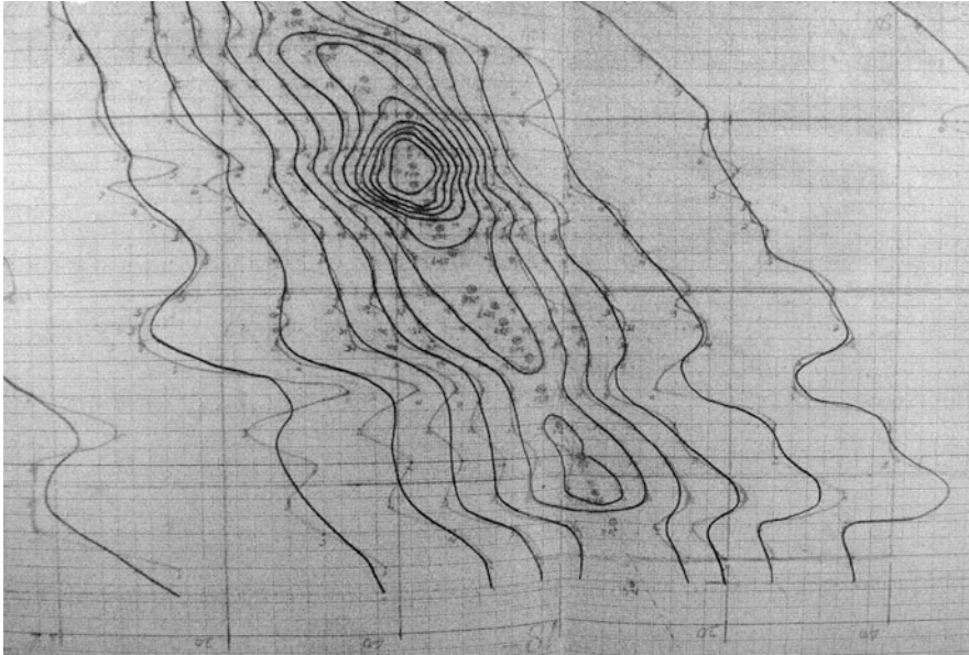
Fig. 23.6 Sgr A region at 400 MHz- beam width 2^\circ . The declination grid is at intervals of about 4^\circ . Dover Heights 80 foot Hole in the Ground antenna. His initial contour image drawn in equatorial coordinates. Constructed late 1953 or early 1954. Credit: Courtesy of the McGee archive in the National Archives of Australia. NAA: C4633/3
