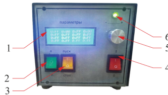
Fig. 9. Control unit: 1 - LSD-indicator of current parameters of FPS sensors; 2 - switch direction of rotation of the drive; 3 - TPG drive driver switch; 4 - switch mode of operation of the drive “manual – automatic”; 5 - speed controller of the drive.
