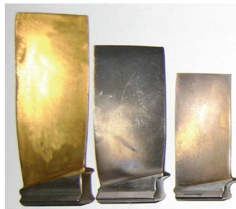
Fig. 6. General form compressor blades of a gas turbine engine model TB3-117.
