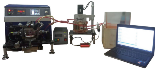
Fig. 3. The complex of devices of comparative estimation of tribological characteristics of commodity oils at the optimization of their current aggregate-phase state.
