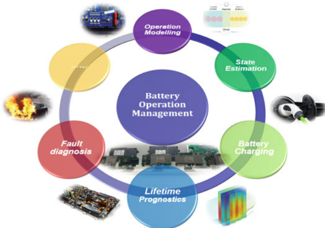
Fig. 2.6 Key tasks of battery operation management
