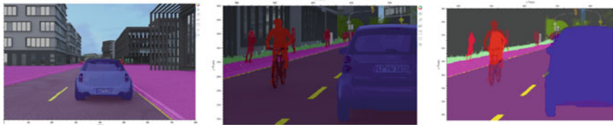
(a) Overlay of input image and ground truth (b) Overlay of ground truth (left) and predictions (right): selected critical images often contain cyclists
