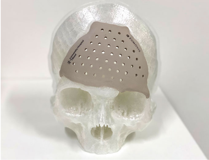
Fig. 4 3D-printed skull implant made of polyetheretherketone (PEEK) (Swiss MAM Research Group, Thieringer, DBE)
