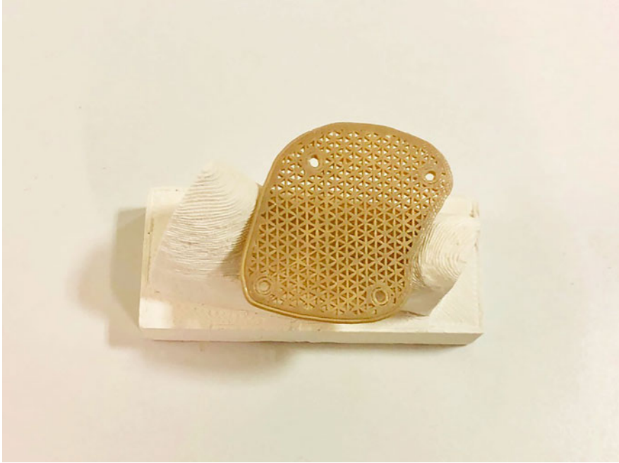
Fig. 5 3D-printed polyetheretherketone (PEEK) shell for guided bone regeneration (Swiss MAM Research Group, Thieringer, DBE)
