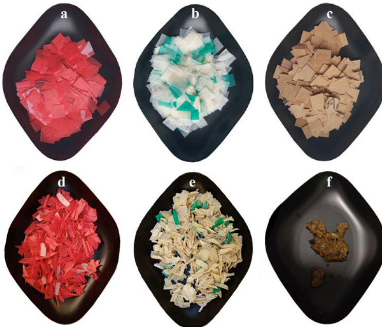
Fig. 4 Pieces fed to semi-continuous tests of bioplastic shopper bag 1—BSB1 (a), bioplastic dedicated bag 1—BDB1 (b), and paper bag—PB (c). Undigested pieces of semi-continuous tests of BSB1 (d), BDB1 (e), and PB (f)
