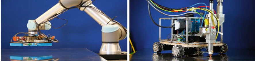
Fig. 1 MVP of a Tool Center Point sensing unit (left), MVP of a mobile robotic system for laser material processing (right)
