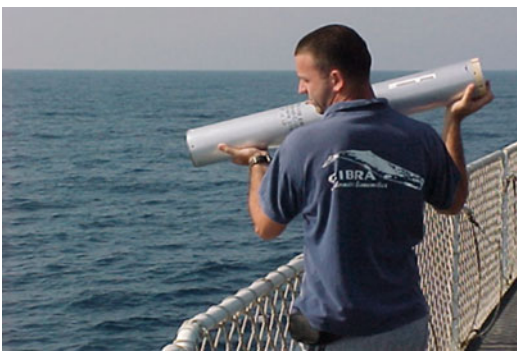
Fig. 2.14 Photograph of a sonobuoy deployed from a ship to monitor whale sounds in the Mediterranean Sea (SOLMAR Project, http://www.unipv.it/cibra/res_solmar_uk.html )
