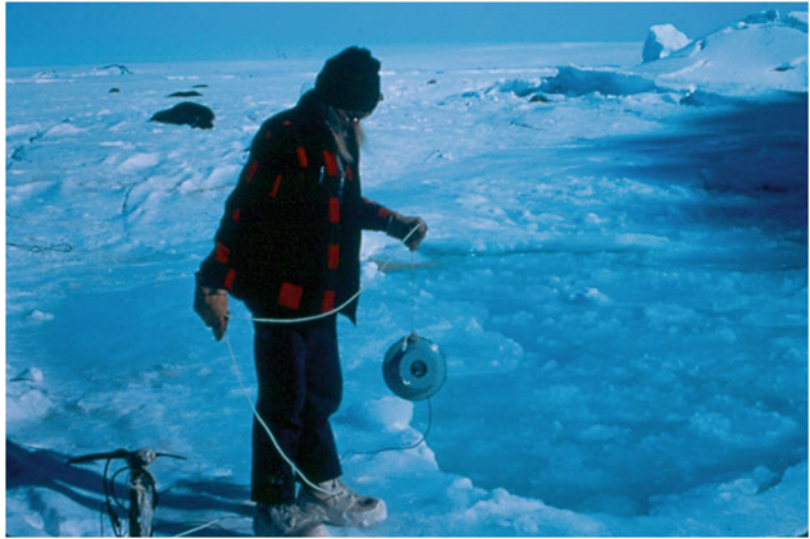
Fig. 2.18 Photograph of JA Thomas lowering a Lubell underwater speaker into a melt hole to play back underwater vocalizations to Weddell seals ( Leptonychotes weddellii ) in the Antarctic
