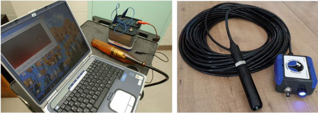
Fig. 2.12 Photographs of an ITC 6050C hydrophone with built-in preamplifier and external battery power (left) and a Cetacean Research Technology C57 hydrophone with cable and battery box (right; courtesy of J R Olson)
