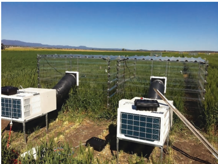
Fig. 10.2 Heat chambers with attached air conditioning units deployed in the field at Narrabri, NSW, Australia
