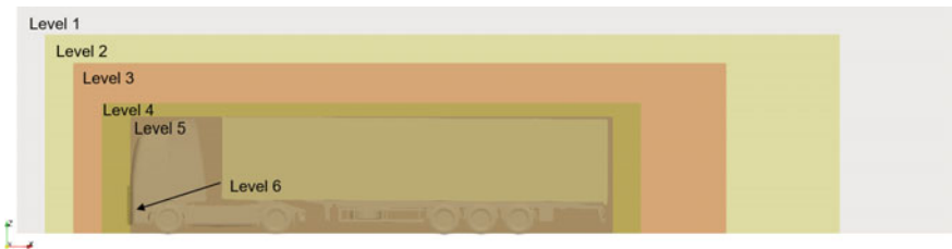
Fig. 5.4 Arrangement of the refinement boxes for meshing
