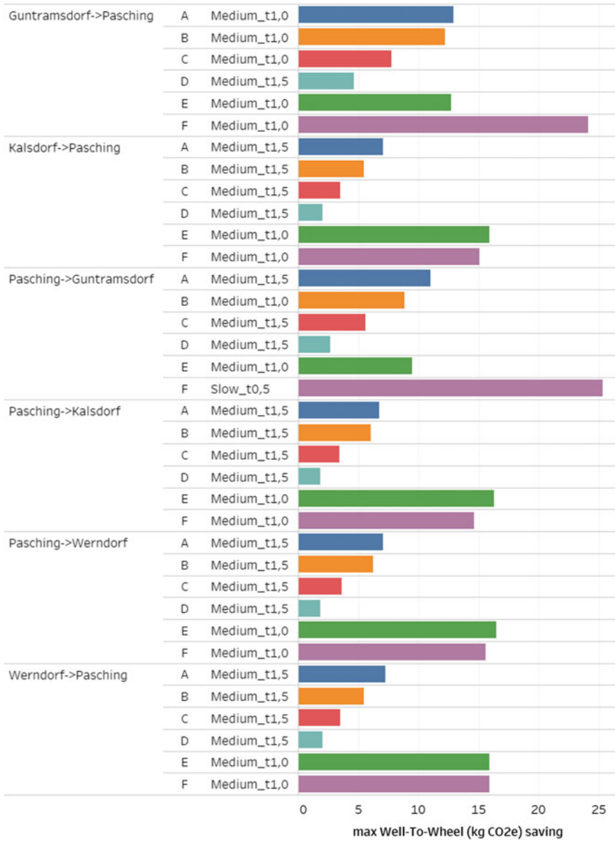
Fig. 12.4 Maximum well-to-wheel savings in 3-truck platoon—fleet operator example
