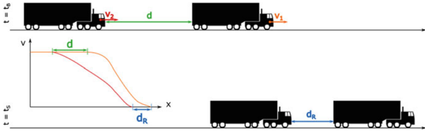
Fig. 9.2 Safe braking within a platoon. Starting from an initial distance d and initial speeds v_1 and v_2 at time t_B , each truck decelerates according to its deceleration capacity. A positive residual distance d_R at time t_S indicates that a collision can be avoided
