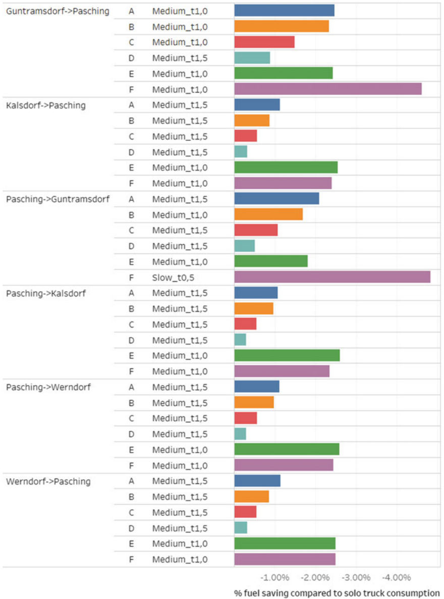
Fig. 12.2 Maximum average fuel savings in 3-truck platoon—fleet operator example
