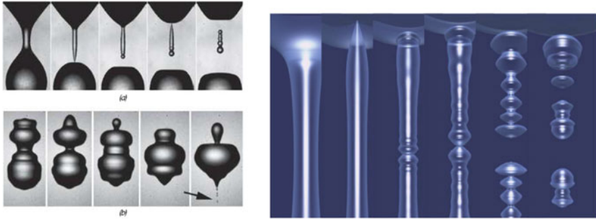
Fig. 4 Droplet dynamics. Left, experiment taken from [41]. Right, level set calculation of surface capillary waves, taken from [12]
