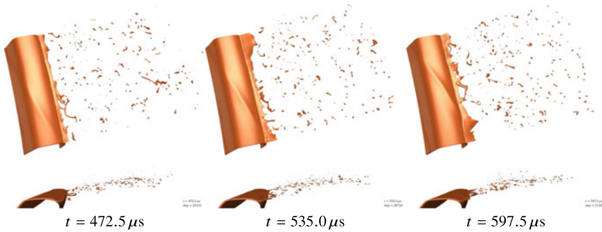
Fig. 13 Three-dimensional model results of rotary bell atomization for time- and spatially-varying inflow film thickness, high mesh resolution, and shaping air currents simulating nozzle inlets. In each of the nine panels, two viewpoints at the same time frame are given: a top-down perspective and a side-on view to show the vertical drifting of the shedding droplets, being pushed upwards by the shaping air currents. The liquid surface is colored copper, with the bell cup situated beneath
