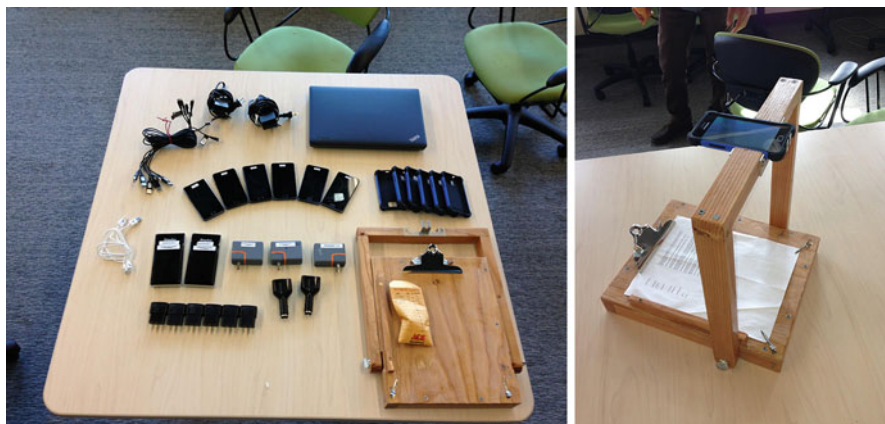
Fig. 15.11 The Open Data Kit (ODK) mobile phone and backup jig to take photos of paper surveys
