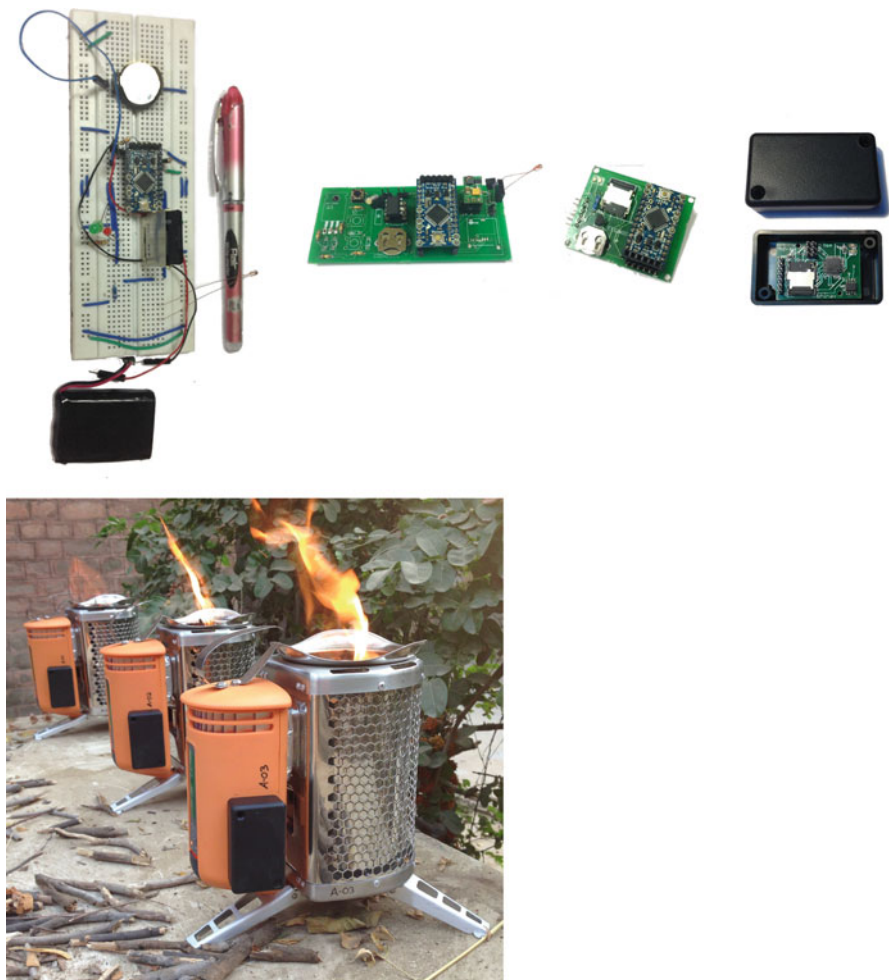
Fig. 15.16 Top: Evolution of the ASUM from breadboard to final manufactured device. Bottom: ASUMs installed on BioLite cookstoves undergoing functional testing at IIT Delhi
