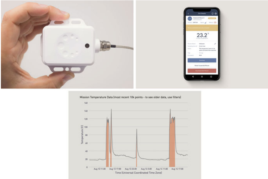
Fig. 15.17 Clockwise from top-left: a Geocene Dot-brand thermocouple data logger, the Geocene mobile application, and a screenshot of temperature time series data with cooking events detected and highlighted from Geocene’s web application, Geocene Studies
