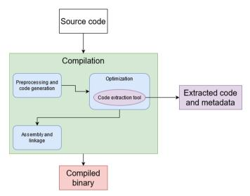
Fig. 3. Simplified compilation process and location of the extraction tool
