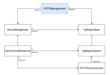
Fig. 4. Extended component diagram for OpenCL operation
