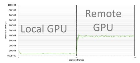
Fig. 6. Response time with a live device swapping for a local to a remote GPU
