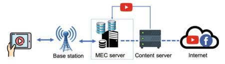
Fig. 4.2 Example application of MEC: video content caching
