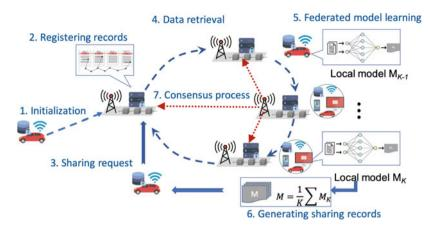
Fig. 4.6 The processes of MEC-empowered model sharing
