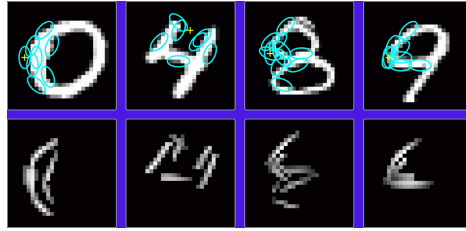
Fig. 2. The configured COSFIRE filters are represented by the set of light blue ellipses in the top row, whose orientation indicates the preferred orientation of the Gabor filter. In the bottom row, the part of the object that the corresponding COSFIRE filter is able to detect (figure from [3]). (Color figure online)
