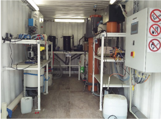
Fig. 6.7 Test room with the anoxic pilot filter system for the downstream denitrification at the Suzhou II wastewater treatment plant
