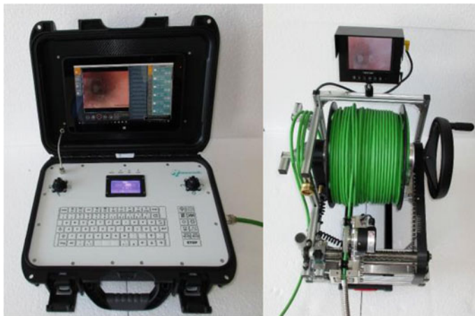
Fig. 7.7 Portable control system (left) and cable drum with integrated video monitor (right). (JT Elektronik)
