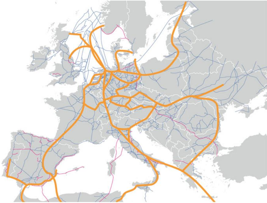
**Fig. 4** Natural gas infrastructure in Europe (blue and red lines) and first outline for a hydrogen backbone infrastructure (orange lines). The main part of the hydrogen backbone infrastructure consists of re-used natural gas transport pipelines with new compressors. A new pipeline from the solar and wind resource areas in Greece needs to be realized
