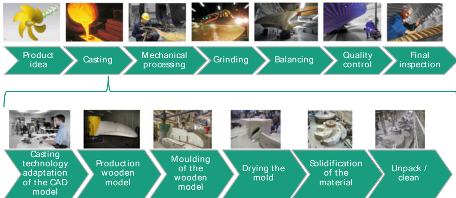
Fig. 1 Conventional production process using the example of a fixed pitch propeller
