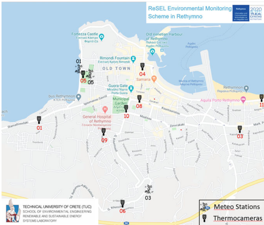
Fig. 3 Meteo stations and thermocameras sites
