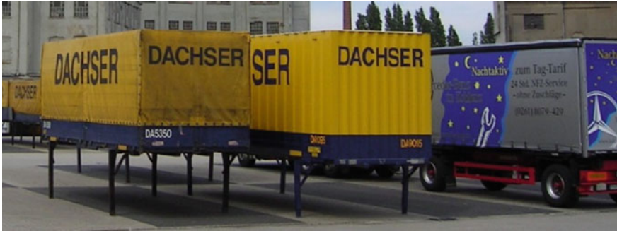
Fig. 1 Exemplary representation of swap bodies used as micro-hubs. Source Dachser Neuss Swap Bodies. Licensed under CC BY-SA3.0 ( https://creativecommons.org/licenses/by-sa/3.0/deed.de ). Cut out. Original version: https://de.wikipedia.org/wiki/Datei:Dachser_Neuss_Swap_Bodies.JPG
