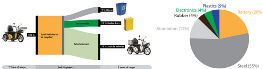
Fig. 13 Majority of the KYBURZ DXPs are refurbished, and those which are recycled result in good yields
