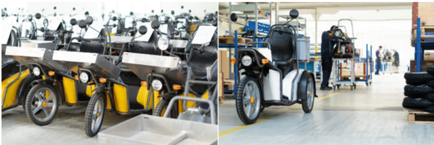
Fig. 12 KYBURZ SecondLife project refurbishment hall and production line
