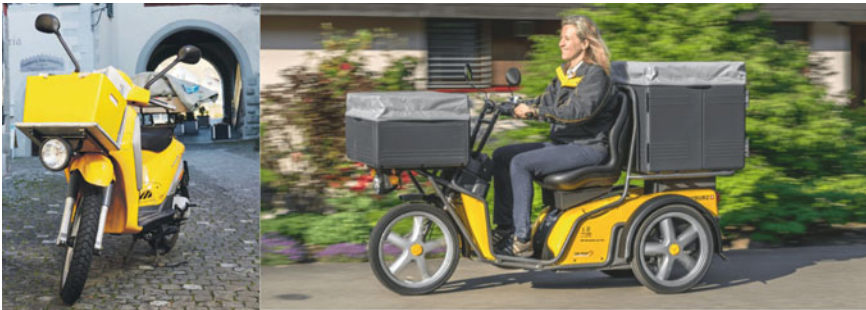
Fig. 4 Piaggio Liberty 125 cc internal combustion engine (ICE) incumbent delivery vehicle (left) and the KYBURZ DXP electric delivery vehicle (right)
