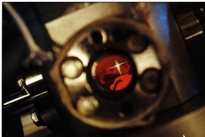
Fig. 9 View through a window into the gain region of the molecular beam laser. The glowing red part is the molecular beam source with a cooler (darker) thermocouple attached. The thin yellow trace marks the pump laser beam which excites also background molecules. The thicker yellow region is seen because of radiation diffusion between particles along streamlines of the molecular beam. The gain region is the crossing between the two yellow traces
