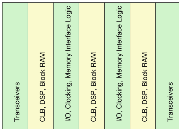
Fig. 3.38 Floor-plan of column-based Xilinx® UltraScale FPGAs
